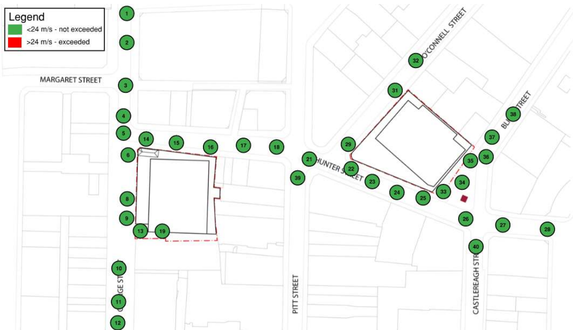
Figure 3-6 Irwin sensor safety results for proposed development
